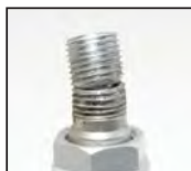
Galvanic corrosion causes TPMS failures.
