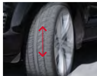
STATIC IMBALANCE: The wheel has a tendency to jump.
