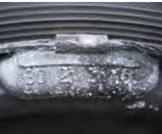
UNCOATED WEIGHTS: Contact corrosion of surface
